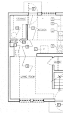
TWO BEDROOM UNIT - TYPE A FIRST FLOOR PLAN - DEMOLITION Scale: 1/4" = 1'-0"
