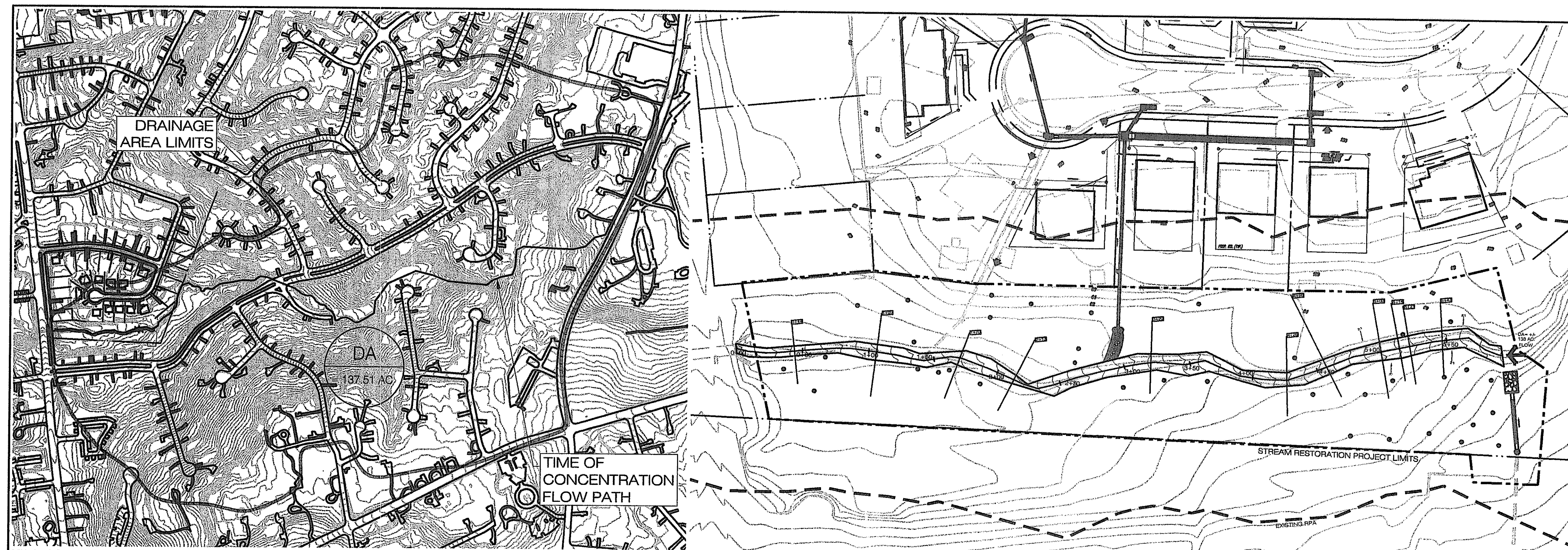
TAFT AVENUE: DRAINAGE AREA SCALE: 1 INCH = 500 FEET
